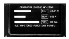
The APD-192G088 is a full field dot matrix display with 192 columns and 88 rows. It includes drive electronics and a microprocessor based controller. The controller maintains all the refresh memory, character generation and control logic with parallel or serial interface and a DC to DC converter to generate the necessary panel voltage. A touch panel version is also available (APD-192G088-5).
